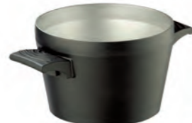
4-l Heating bath for oil Max. temperature 250 °C P/N 036110390
