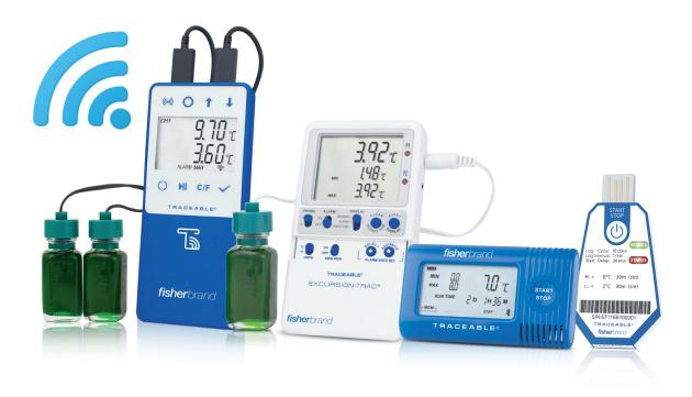
The Fisherbrand™ series of Traceable Temperature Dataloggers provides an accurate and reliable multi-point record of temperatures and other environmental measures over time to help monitor quality and output. They are widely used in many research and academic laboratories, and food processing, medical, agriculture, and environmental work environments.
