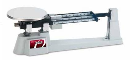
**If the beam still sticks:** It is possible the Damper Vane is bent. To correct this, follow the instructions for removing the Trig Loop Assembly. Once the Assembly is removed, use needle nose pliers to straighten the Damper Vane.
