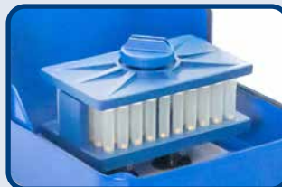
TallFlex™ Adapter 48 x 4.5 mL tubes Cat. No. MP116010580
