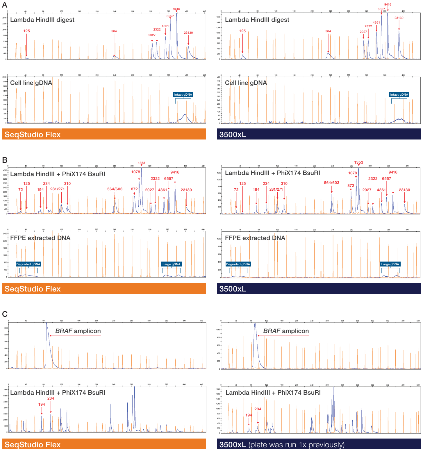
Figure 4. Analysis of double-stranded DNA by CE. (A) Different DNA preparations were electrophoresed through capillaries containing POP-7 polymer at reduced temperature. Single-stranded LIZ-labeled fragments were included in the capillary. Lambda HindIII digest fragments and genomic DNA from A549 cells were analyzed in different capillaries. Note the typical pattern of lambda fragments (top panels). These can be used to estimate the size of the gDNA population of about 9–23 kb (bottom panels). Equivalent performance was seen on both instruments. (B) A mixture of lambda HindIII and phiX174 BsuRI digests and DNA extracted from an FFPE tumor sample were analyzed in different capillaries. Note the typical pattern of phage fragments (top panels); these can be used to estimate the size of the fragmented DNA (75–190 bp) and the large genomic DNA (bottom panels). Equivalent performance was seen on both instruments. (C) An amplicon containing the BRAF V600E region was analyzed before cycle sequencing, along with a mixture of lambda HindIII and phiX174 BsuRI digests in different capillaries. Note the typical pattern of phage fragments (top panels); these can be used to estimate the size of the BRAF amplicon (194–230 bp). This is very similar to the expected size of 208 bp. Equivalent results were seen on both instruments.
