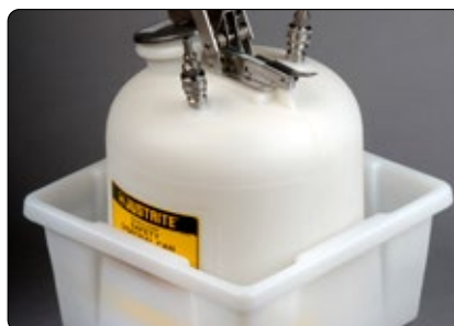
Spill Basin captures inadvertent leakage from HPLC inflow tubes
