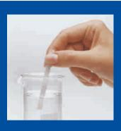
2. The reaction zones are wetted with the solution to be tested simply by dipping them briefly into the liquid sample. Any excess liquid is then shaken off or removed by drawing the test strip across the edge of the vessel.
