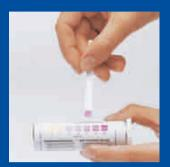
**3.** After the specified reaction time of at most one minute has expired, the color of the reaction zone is compared with the color scale printed on the tube label and the corresponding concentration is read.
