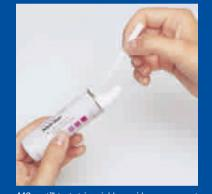
MQuant<sup>™</sup> test strips yield a rapid measurement result in the semiquantitative range for over 30 parameters.
