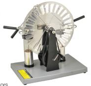
constructed from Corning glass and aluminum foil. This Wimshurst is mounted on a sturdy ABC base, stands 38 cm tall, and can generate up to 75,000 volts. User manual included.
